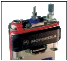
Multiple silicon seals protect the radio from water and foreign particles.
